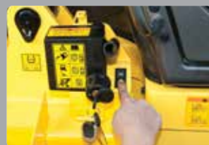
Cabin tilting automatic system Cabin tilting automatic system makes servicing of all power train components quick and easy. An electrically assisted hydraulic actuated cylinder tilts operator cabin to left side about 54 degrees for easy access to inside of truck components.
