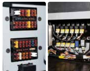
Compact fuse box for easy inspection
